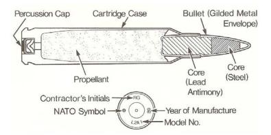
All ammunition issued for this weapon is rimless; its calibre is 5.56 mm and this, together with manufacturing information, is stamped on the base of each cartridge.
