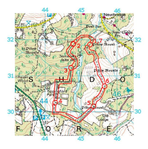
Distances should be calculated using the grid squares (the distance between Northings or Eastings is 1Km).
